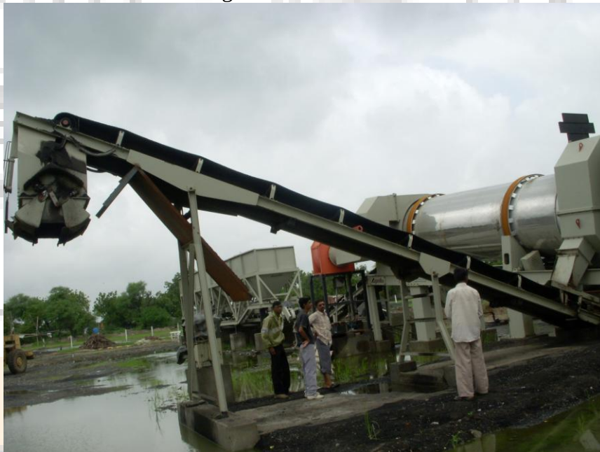
Fig. Load Out Conveyor
