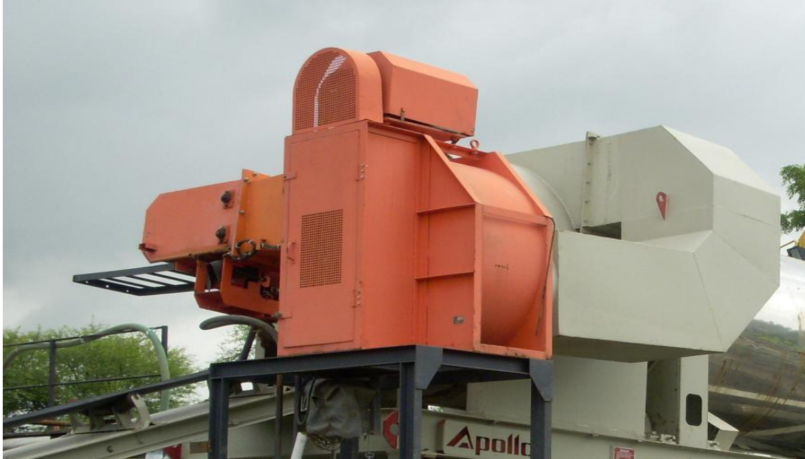
Fig. Aggregate Dryer
